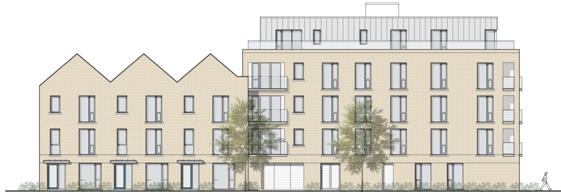
Image 12. Elevation showing Block A at the Main Street, buff two tone brickwork with zinc cladding to the penthouse level.
