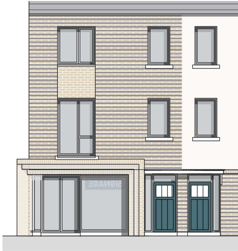
Image 6. Elevation showing the setback horizontal brick detail to the Southern Side of Main St.
