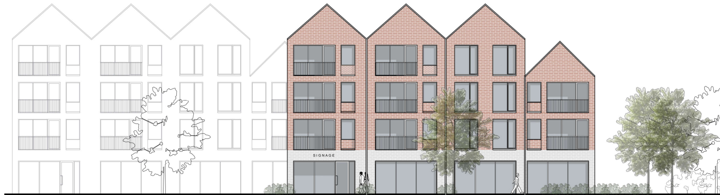
Image 9. Elevation block D at the Civic Plaza on the Main Street red and charcoal bricks with dark metal balustrades to balconies.
